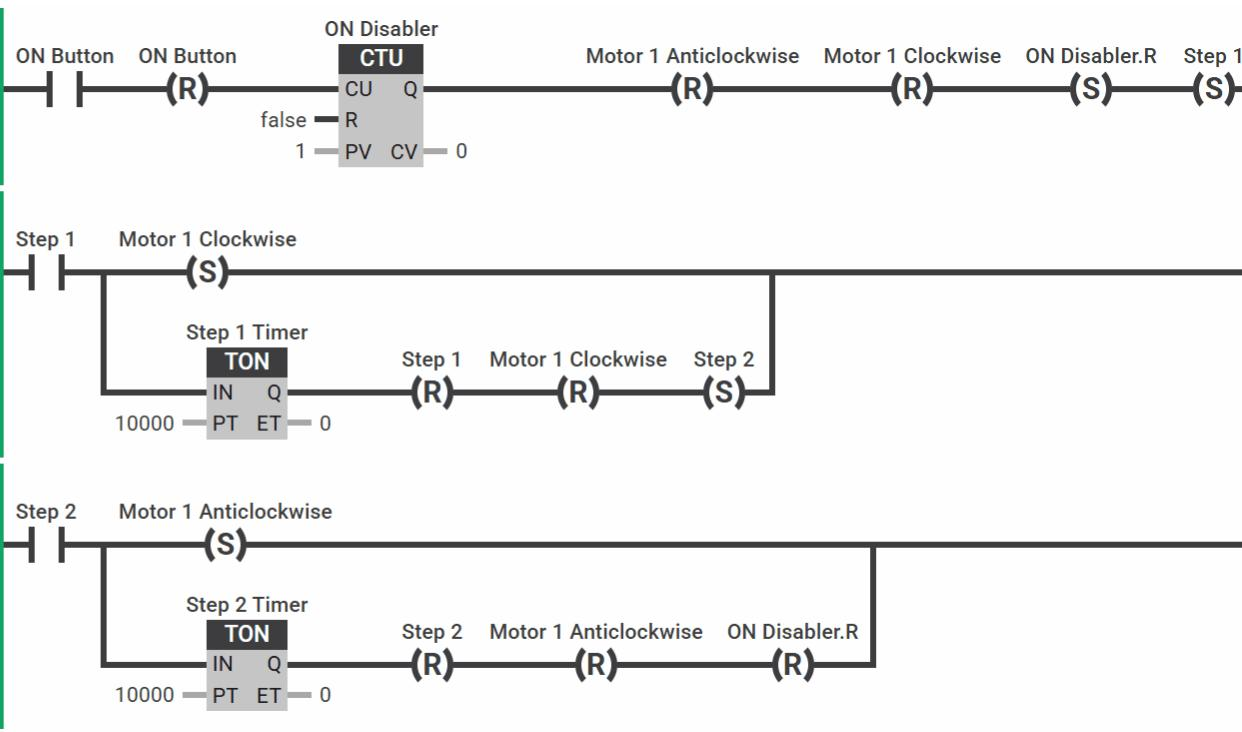
This line controls the turning on of the program enabling Step 1 at the end
