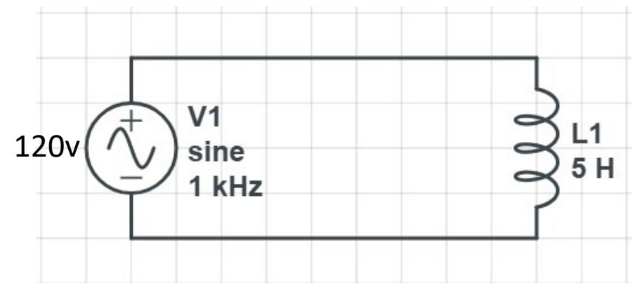
$$\begin{aligned}X_L &= 2\pi f L \\X_L &= 2\pi * 1000 * 5 \\X_L &= 31415.92654\end{aligned}$$
